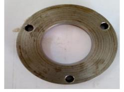
FIG.9: BLANK HOLDER IV. EXPERIMENTAL PROCEDURE
