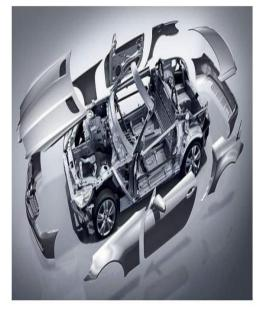
Fig-2 AUTOMOTIVE PARTS PRODUCED BY SHEET METAL FORMING
