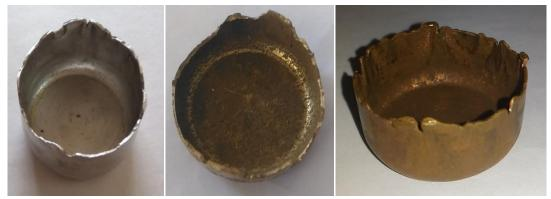
FIG-12: DRAWN CUP FROM THE AL 1100, COPPER AND BRASS
